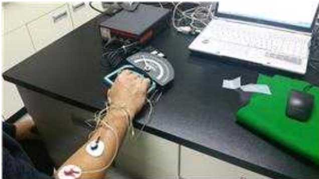
Fig. 2. Measure grasping power with EMG.
